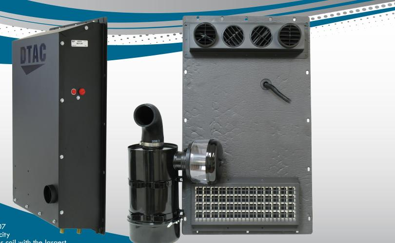
designed for the mining industry, our 807 combines a high capacity evaporator and heater coil with the largest blower assembly available with our systems. Externally mounted, the 807 frees up valuable space inside that would be used by a traditional A/C system. Complete with bolt on pressurizer and Donaldson external filter.
